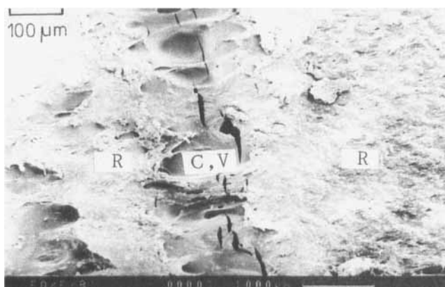
FIGURE 11 SEM photomicrograph showing peel front for carbon black filled adhesive. (R, Rubber; C, V, Cracks and Voids on peel front).
